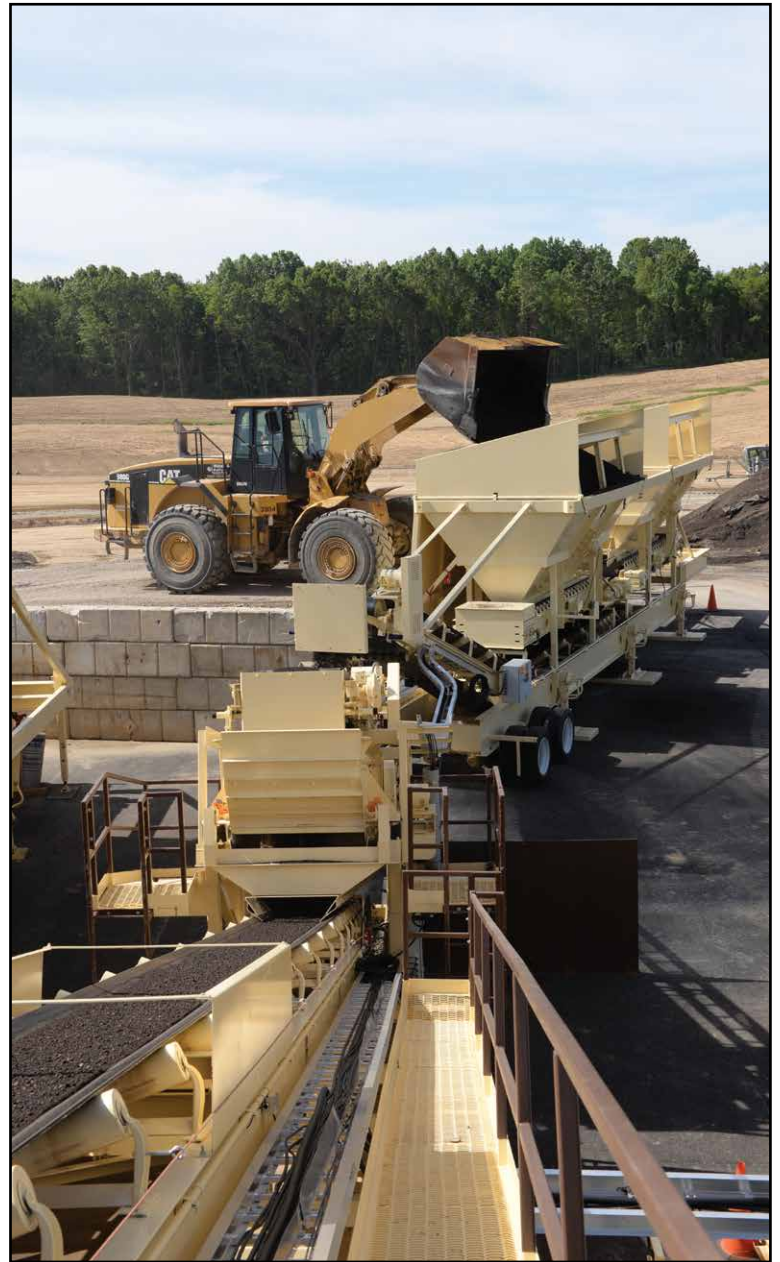
The La Porte plant features a portable 10 ft x 14 ft (3.05 m x 4.27 m) dual bin recycle feed system and a 36 in (91.44 cm) collecting conveyor.
